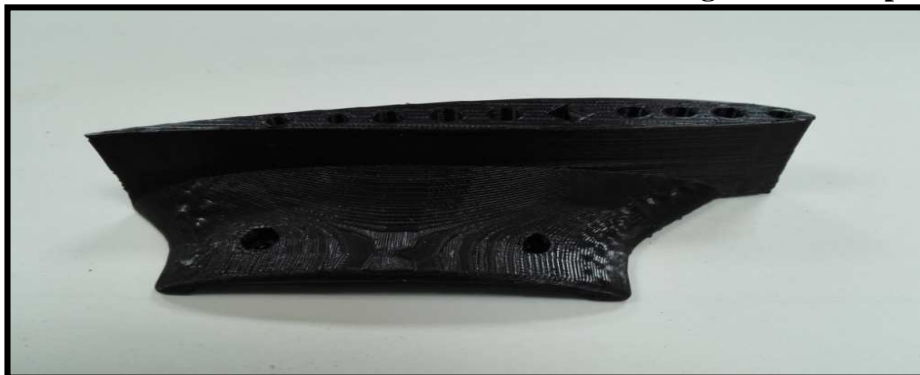
Figure No.11: The manufactured wing-center-link part by Flash forge FDM printer
